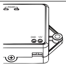
Note: pay attention to the polarity of power input and connect power according to the interface instruction.
