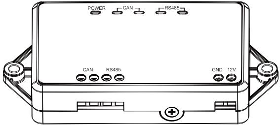
CAN communication interface: It is connected to air conditioner through twocore connection wire, to realize communication between Modbus Gateway(Mini) and air conditioner.
