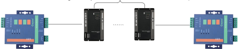
30 Modbus gateways in maximum between two repeaters
