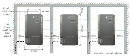
Warning! Power cord and communication line of BACnet gateway must conduct routing separately(the distance shall be over 15cm); otherwise, it might lead to BACnet gateway communication malfunction!
