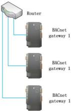
(2) Communication connection between BACnet gateway and AC units (n is the quantity of ODU system, n ≤ 16);
