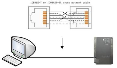
Adopt parallel network cable, BACnet gateway shall go through router to connect to PC.
