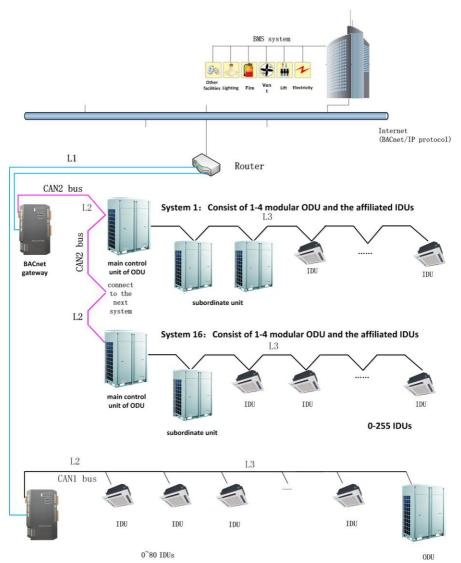
Note: L1 is the standard network cable, L2 and L3 is the twisted pair line.
